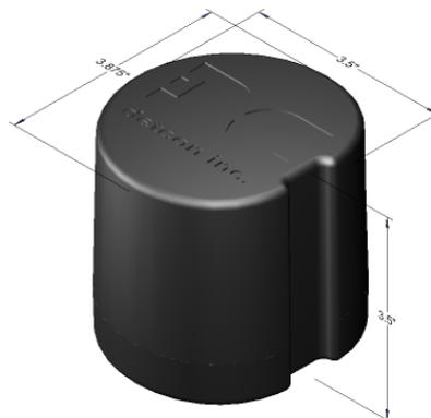
Figure 5 Smart Battery Pack
