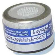
Figure 2 Plug-in Detector
