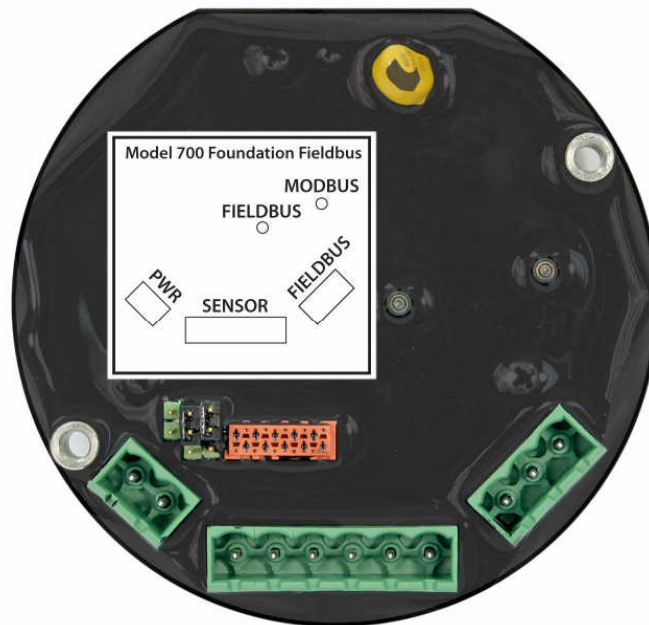
Figure 1 Foundation Fieldbus Bridge PCA
